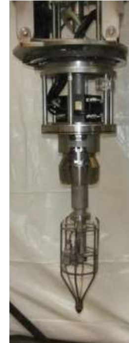
Equipment to sever the inner flange
