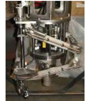
Equipment to sever the outer nozzle
