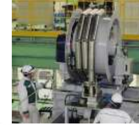
Access equipment for the opening of reactor internals
