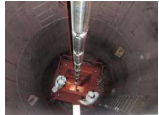
Platform for the mock specimen (inside the test tank)
